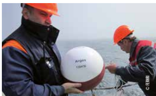
The Argos Tristar buoys are launched from a research vessel by a team of scientists/engineers. The buoys are tethered to the research vessel until the drogue completely submerges.
