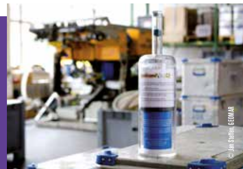
Figure 2. The modern-day message in a bottle, designed by GEOMAR, complete with an Argos transmitter to track the bottle’s path.
