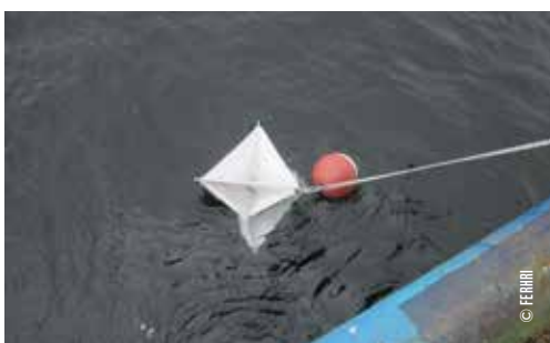
Buoys are connected to the ship as the drogue was not completely submerged.
