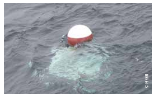
Once the drogue is under water, the tether is removed and the buoy begins its voyage.
