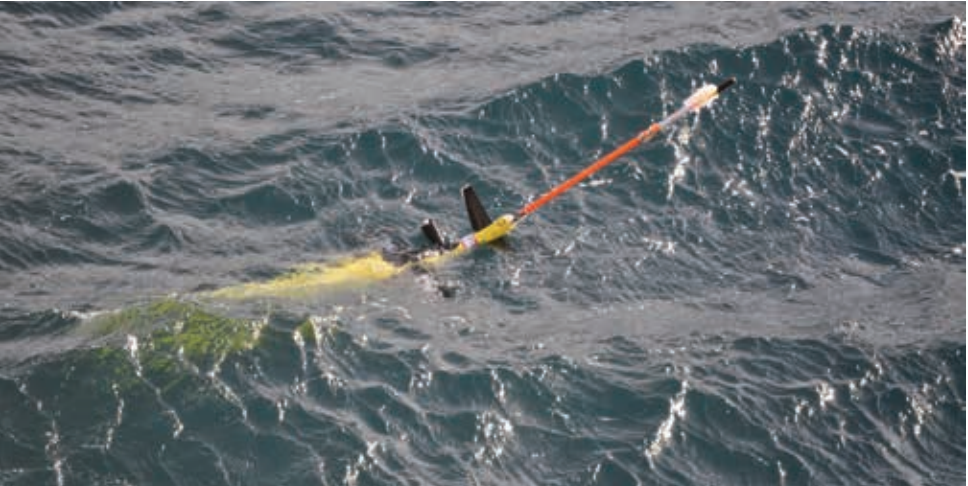
The Seaglider found with the Argos goniometer in February 2014. A block of ice had formed on the sea glider’s antenna, stopping communication with the Iridium system.
