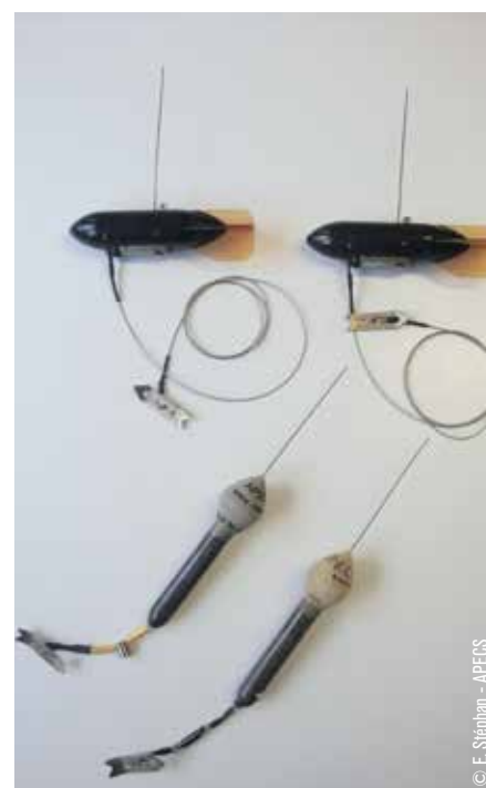
▲ Figure 1: Argos satellite tracking tags by Wildlife Computers that can be attached to basking sharks. The MK-10 archival tags (below) record data underwater for several months before releasing and rising to the surface to transmit data. The towed SPOT tags (above) transmit data whenever the animal rises to the surface.
