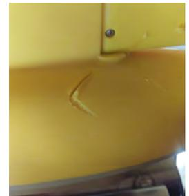
Figure 7: Excellent impression of shark tooth on glider digifin
