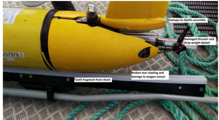
Figure 5: Photo showing the external damage received during shark attack.
