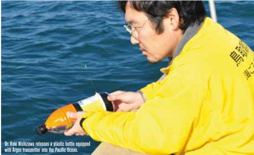
Dr. Koki Nishizawa releases a plastic bottle equipped with Argos transmitter into the Pacific Ocean.
