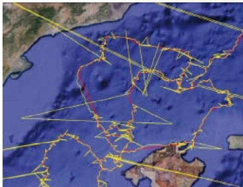
Figure 1 (left) A drifting buoy tracked for 6 months. The GPS tracks are in red, the Argos positions from the current processing system are in yellow.
